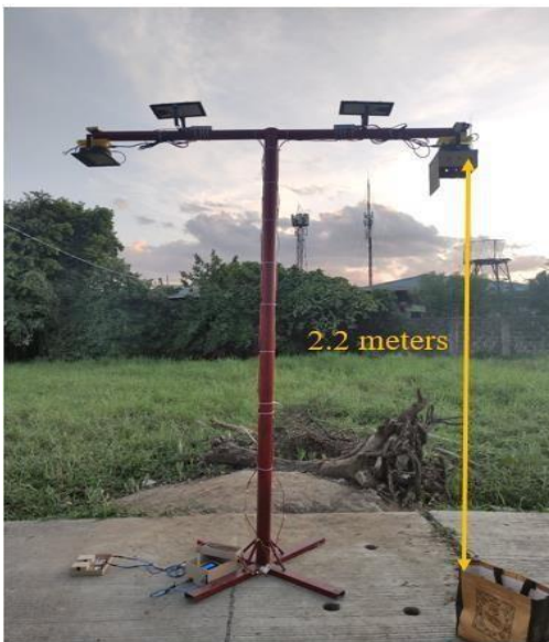
Figure 3.2 - Mounting Height of the Pole
